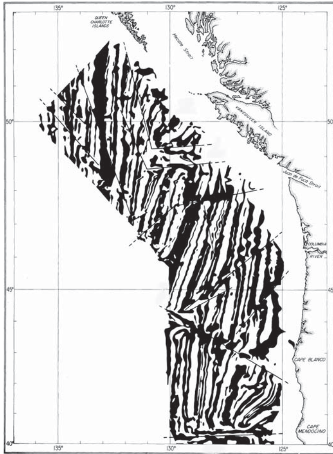
Figure 15.3: Map of the pattern of magnetic anomalies off northwestern North America. [Modified from Mason and Raff, 1961.]
