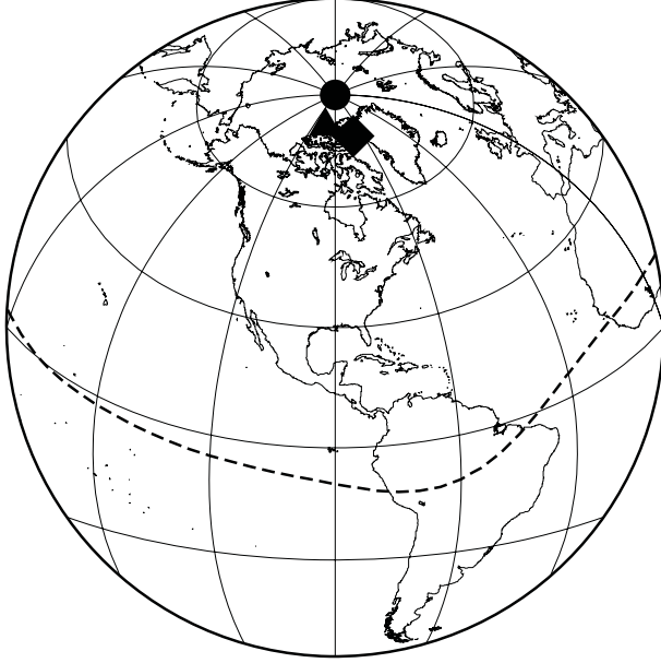
Figure 2.7: The different magnetic poles. The triangle is the magnetic North Pole, where the magnetic field is straight down ( I = +90^\circ ). The diamond is the geomagnetic North Pole, where the axis of the best fitting dipole pierces the surface. The dot is the geographic North Pole. The dashed line is the magnetic equator where I = 0^\circ .
