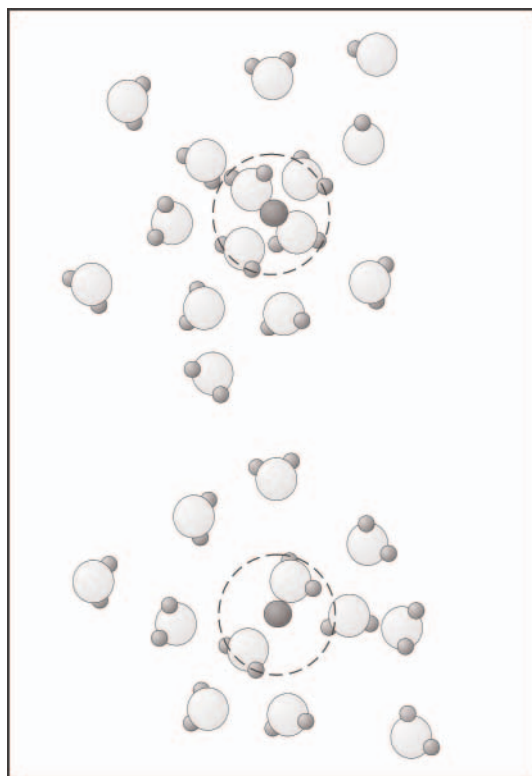
FIG. 10. A sketch illustrating the statistical nature of hydration shells (large dashed open circles) forming around molecules of an inner sphere complex (MeCl) indicated by the dark solid circles. The upper molecule is surrounded by four water molecules, whereas the lower molecule only has two water molecules in close proximity. Based on this diagram, the average number of water molecules surrounding molecules of the inner sphere complex (MeCl) is three and thus the statistical hydration number of the species is three.
