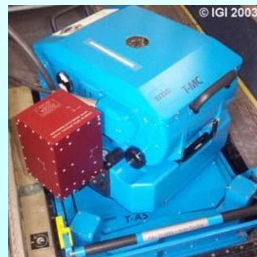
System installation AEROcontrol test IMU-IId mounted at RMK-Top camera
