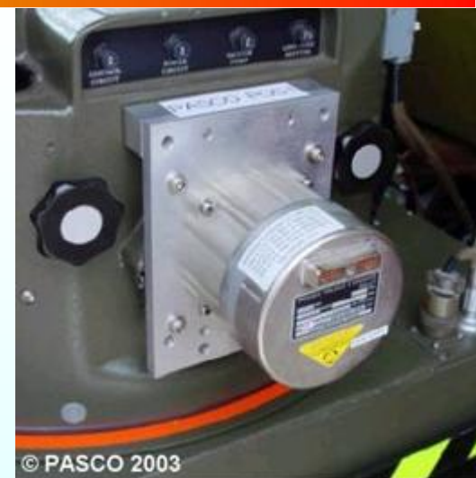
System installation POS/AV test LN200 IMU mounted at RC30 camera
