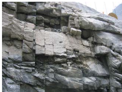
(c) 左岸顺坡向卸荷裂隙
