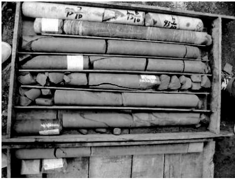
图2 矿体及顶板围岩(ZK1908 钻孔岩心) Fig.2 Orebody and surrounding rock in roof (cores from borehole ZK1908)
