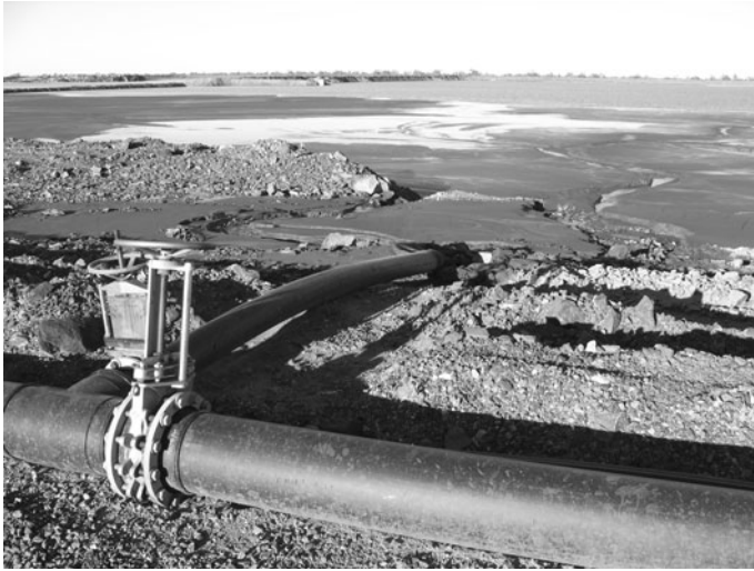
Fig. 4.4 Discharge of tailings from a spigot pipe into a tailings storage facility, Cannington silver-lead-zinc mine, Australia
