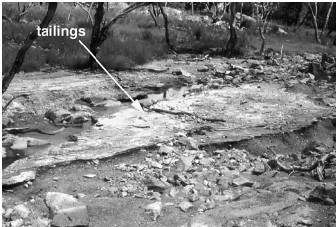
Fig. 4.13 Sulfidic tailings layer in ephemeral creek bed downstream from the derelict lead-zinc Webbs Consols mine, Australia. The tailings contain wt.% levels of arsenic, lead and zinc
