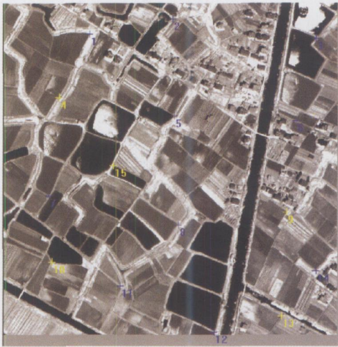
图 7 传统方法选取的控制点分布 (黄色:检查点,蓝色:控制点) Fig. 7 Control points selected manually (the yellow are check points and the blue are control points)
