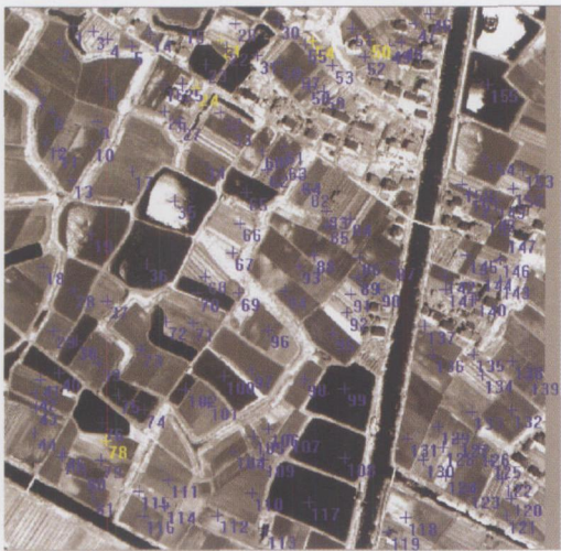
图 6 本文方法自动提取的控制点分布 (黄色:检查点,蓝色:控制点) Fig. 6 Control points generated by the new method (the yellow are check points and the blue are control points)
