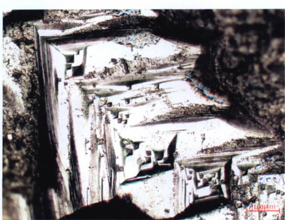
图 4 微分干涉显微镜高倍率下“十字架”线条为由大量大小不等的正方形 腐蚀坑沿[100]方向折重叠排列而成(100×) Fig. 4 Microphotograph showing the “cross” dissolution pattern consisting of a large number of tiny square-shaped etch pits in [100] direction
