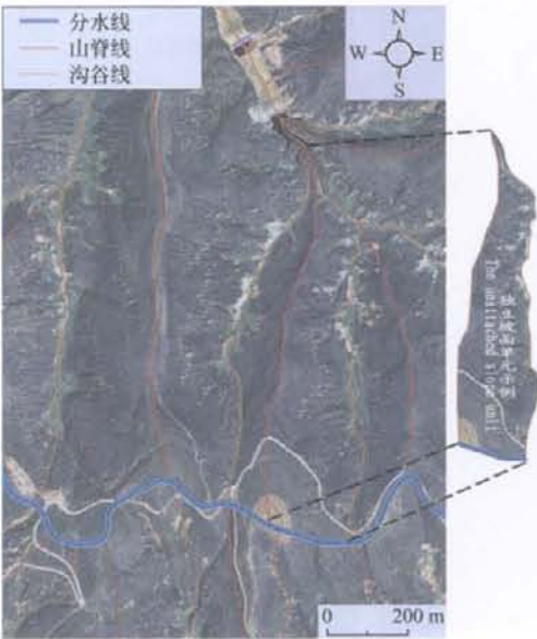
图3 利用分水线、山脊线和沟谷线划分的独立坡面单元 Fig.3 Unattached slope units divided by watershed line, ridge line and valley
