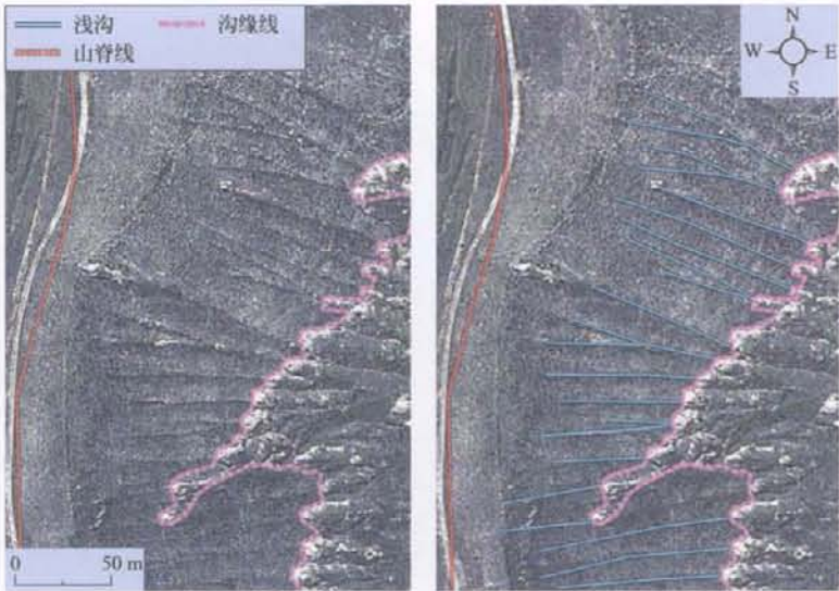
图4 独立坡面单元内的浅沟勾绘示意图 Fig.4 Schematic of ephemeral gullies in unattached slope unit
