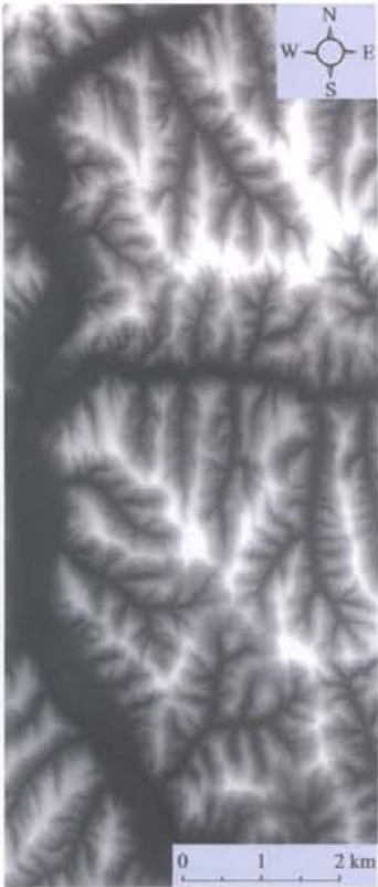
图2 研究区5 m分辨率数字高程模型(DEM) Fig.2 DEM of 5 m resolution in study area
