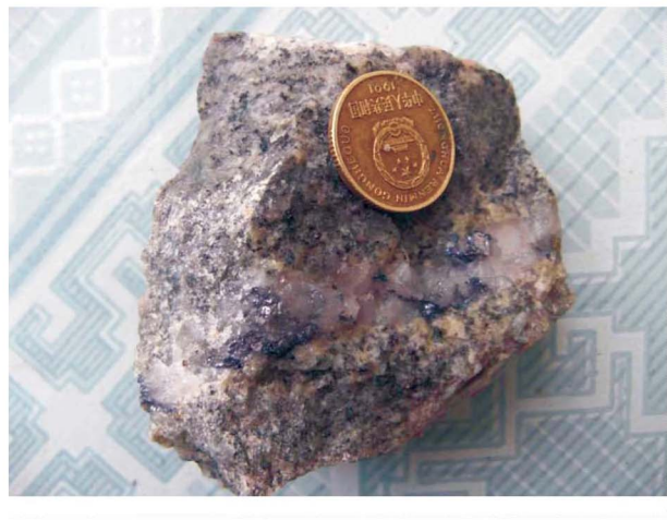
图 3 德保铜锡矿床内含黄铜矿石英脉中的辉钼矿 Fig. 3 Molybdenite aggregates in a chalcopyrite-quartz vein from Debao Cu-Sn ore deposit
