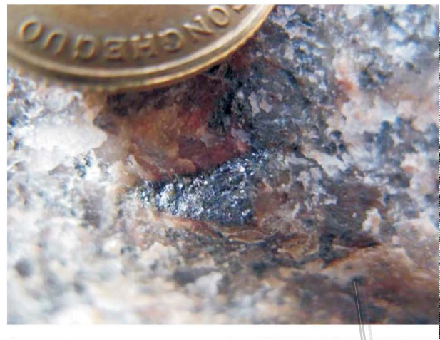
图 4 德保铜锡矿区花岗岩中浸染状辉钼矿 Fig. 4 Disseminated molybdenite in granite from Debao Cu-Sn ore district
