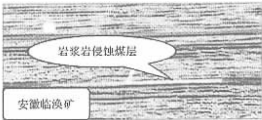
图5 岩浆岩侵蚀地质现象在时间剖面上的显示 Fig.5 The display erosion of igneous rock, coal flushed zone, interlayer rock thickness in seismic time section
