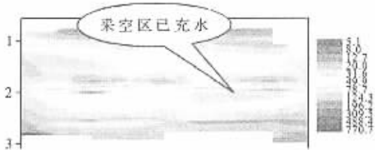
图2 采空区及其含水性在时间剖面及电性剖面上的显示 Fig.2 Display of mined-out area and its water-bearing character in seismic time section and electrical profile
