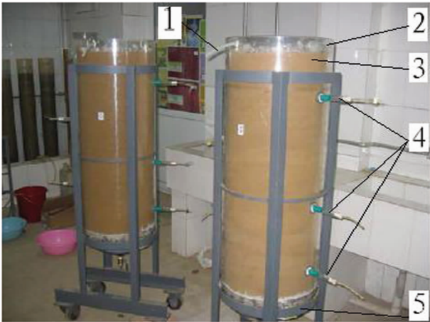
图 1 土柱试验装置图 1—溢流孔;2—有机玻璃土柱;3—试验土样; 4—取样管;5—支架 Fig.1 Test device of soil column 1—Overflow hole;2—Plexiglass soil column; 3—Test soil;4—Water sample tube;5—Support
