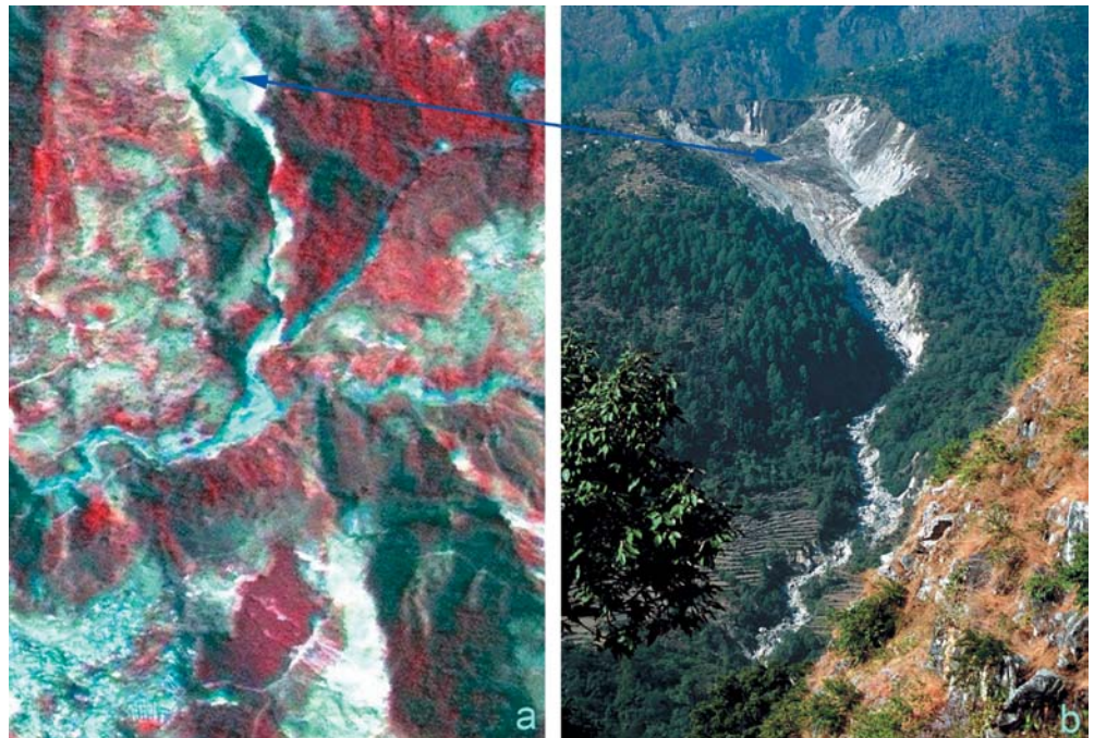
Fig. 2 A typical landslide as identified from a IRS-PAN image and b the corresponding field photo (indicated by arrow)
